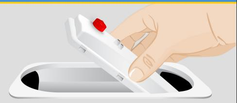
The TIS500A core can now be clipped into the base by first inserting the two tabs at the connector end of the core into the base and then clipping the tab on the opposite face as shown.
