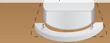
The base is held against the ceiling using the two semi-circular brackets.
