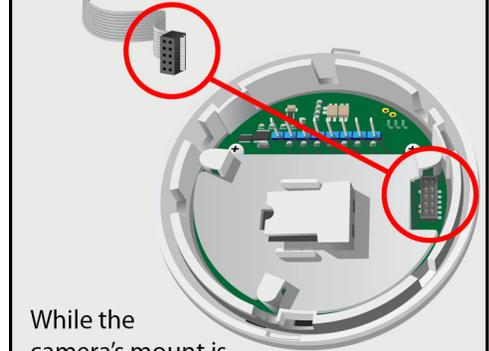
While the camera's mount is on the ceiling, we need to connect a Female 10 Pin IDE Cable with Female DB9 Port on the other end before programming the device with the use of a laptop or computer.
