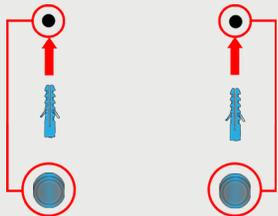
Insert the screws in the JBox's mounting holes, and mount the JBOX on the wall.
