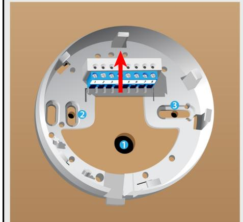
Once the position is determined, we can now drill all necessary holes. Hole #1 is intended for Cat5, Holes #2 and #3 are intended to mount thermal to the ceiling. The arrow in this illustration goes inside the store, so make sure the device is properly positioned.
