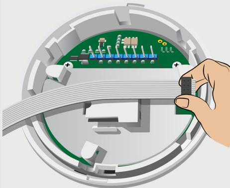
Plug the DB9 / 10 Pin IDE Cable to the specified port.
