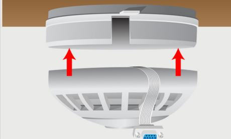
When the DB9 / 10 Pin IDE Cable was connected, mount the camera's face on camera's mount which is already mouted on the ceiling. Make sure the cable runs on the space provided on the camera's mount so that the cable will not be a obstruction when locking the thermal device.
