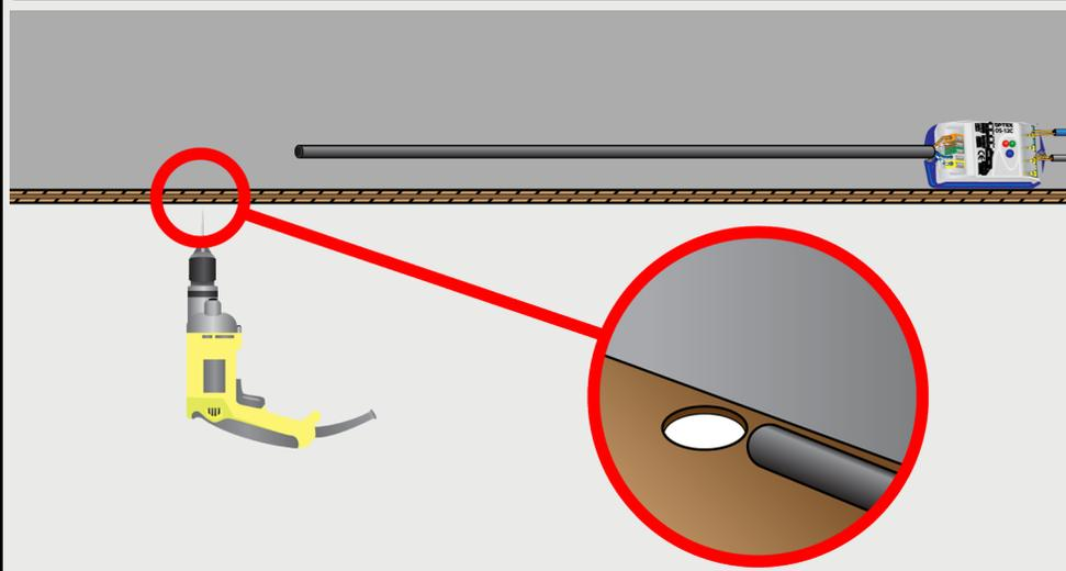
Confirm location of where JBox will be located with Tech Support, (usually near the network switch). Pass cable accordingly, along with other data cables or through conduit.
