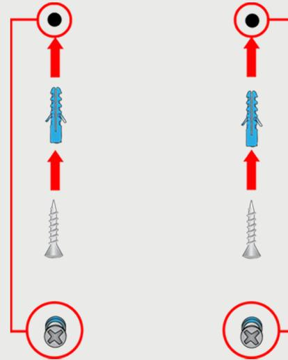
Once the holes are drilled for RTC9000, insert the wall anchors and screw in the first and second holes.
