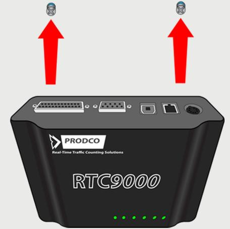
Mount the RTC 9000 on the wall with the use of the screws and wall anchors.
